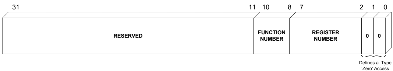
Figure 3-1 Contents of the AD Bus During Address Phase of a Type Zero Configuration Access
